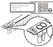
Enter the cartridge code and execute the program. The cartridge code is displayed on the prepacked reagent cartridge and the cover of the manual.
