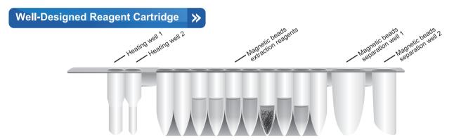
The special shape design of the wells ensures that the beads are fully mixed with the samples and that the washing buffer can be completely drawn up to prevent the remaining of impurities. The reagents required for the experiment have been pre-packed in the reagent cartridge and the cartridge is sealed to avoid contamination.
