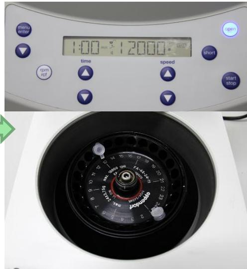
Centrifuge at 10,000 rpm (~11,500×g) for 1 min.
