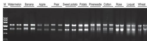
Total RNA purification from watermelon, banana, apple, pear, sweet potato, potato, pine needle, cotton, rose, loquat and wheat with RNAprep Pure Plant Plus Kit, detecting with 1% agarose gel electrophoresis.
