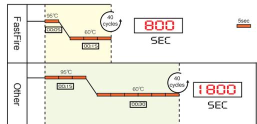
Fig.1 FastFire qPCR PreMix (Probe) uses antibody-modified anti-Taq DNA polymerase, combined with unique fast buffer system, which saves up to 1000 seconds per experiment, improving the experimental efficiency and extending the service life of qPCR instrument.
