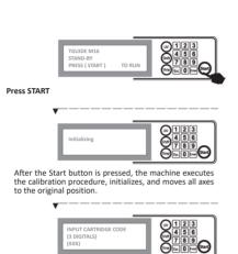
Enter the cartridge code and execute the program. The cartridge code is displayed on the prepacked reagent cartridge and the cover of the manual.
