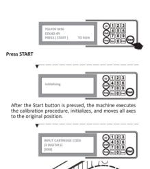
Enter the cartridge code and execute the program. The cartridge code is displayed on the prepacked reagent cartridge and the cover of the manual.
