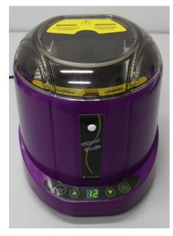
Use a plate centrifuge to briefly centrifuge N96 well plate or 8-tube strip. Please note to make the bottom of the plate outward and keep balance.
