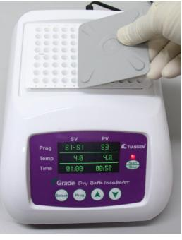
When using the 8-tubes strip, cover the tube cover and compact with a capper after prepared and sub-package of the reaction system. Mark on both ends of the tube cover. Don't mark the tube cover directly above the detection well, or it will affect the fluorescence reading.
