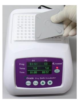
When using the 8-tubes strip, cover the tube cover and compact with a capper after prepared and sub-package of the reaction system. Mark on both ends of the tube cover. Don't mark the tube cover directly above the detection well, or it will affect the fluorescence reading.
