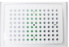
5. Divide the mixture into each detection tube/well, and add the samples in the order of mixture-template- $ddH_2O$  (if necessary) to prepare the system and thoroughly mix evenly.
